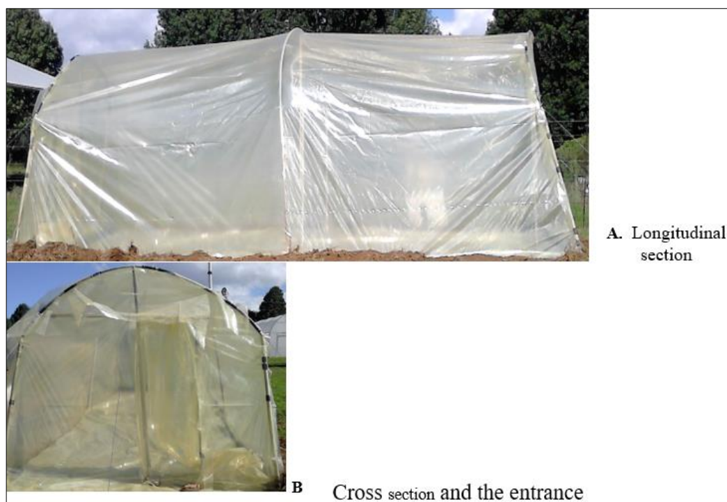
Fig 1: A tunnel solar dryer used in the drying of peach leather products (A, Longitudinal; B cross Section)
